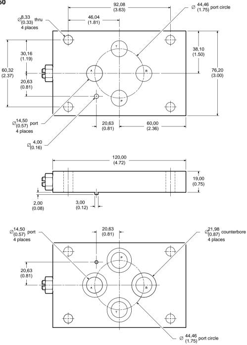
**NOTE** Viton port O-rings (AS568-018) provided: 1,78 (0.070) cross section and 18,77 (0.739) inner diameter.
